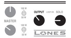
Should you ever use your **LONE STAR** amplifier as a power amp alone by inserting a signal into the RETURN jack, the **OUTPUT** control will serve as the master level control.
